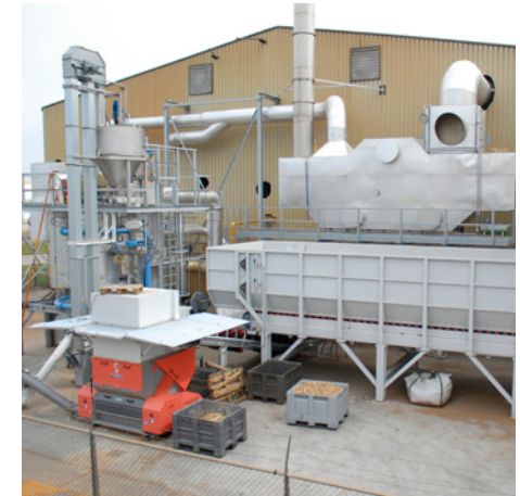
Above: 3.5MWth Waste Wood Gasifier.
