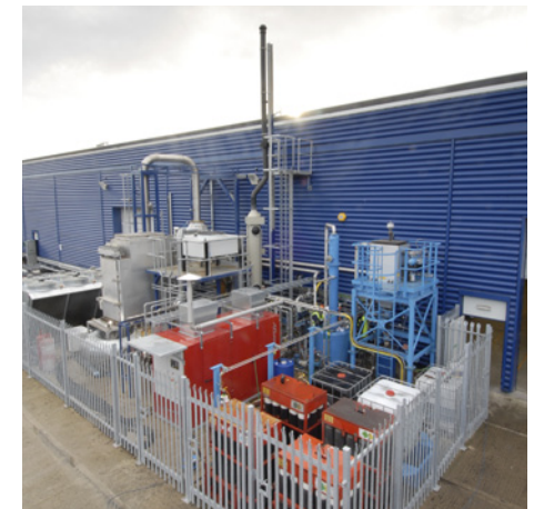
Above: Advanced Plasma Power Gas plasma scale version of 11MWe net output power island.
